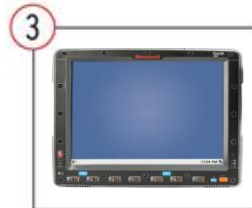
3 Staplerterminal: WLAN-Anbindung an LVS
